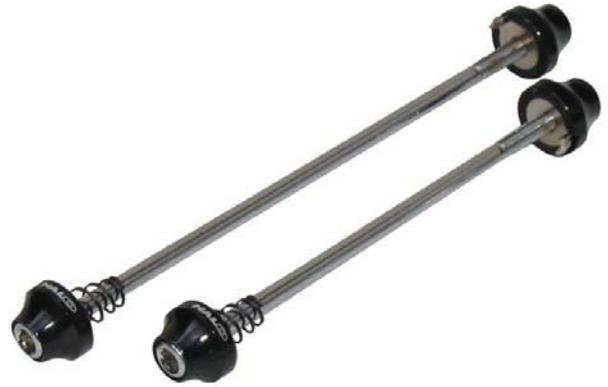
We are concerned that if the instructions were followed literally at such an unnecessary high level of torque as equivalent to 9.5Nm, this could cause additional stress to the rod, and therefore may encourage premature skewer rod failure. If the rod snaps, it has the potential to release the wheel from the bicycle without warning and therefore could cause a serious injury.
